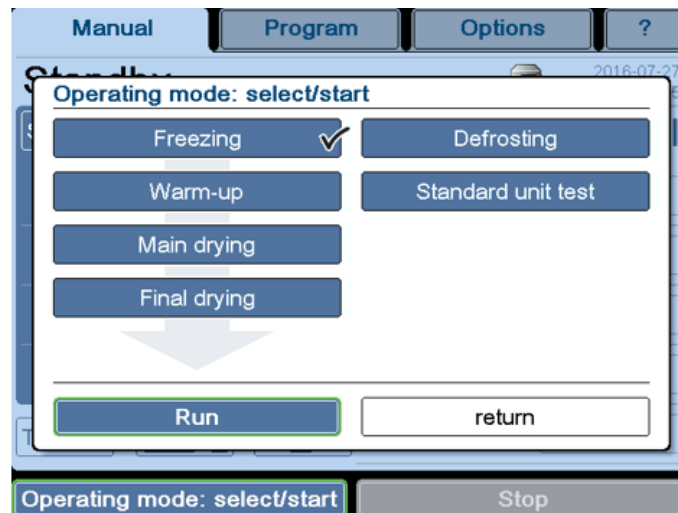
Fig. 29: Dialog box "Operating mode: select/start" (The version of the dialog box that is displayed depends on the equipment of the freeze-dryer.)
