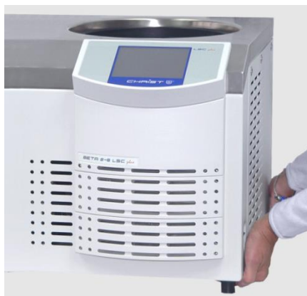
Fig. 10: Lifting the freeze-dryer
