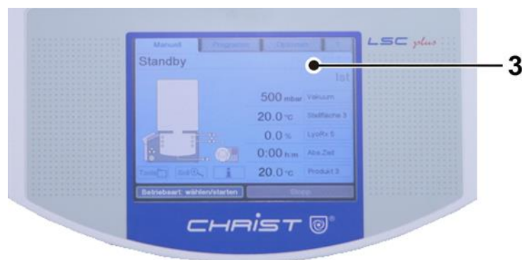
Fig. 2: User interface with touchpanel
