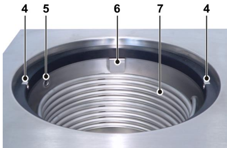
Fig. 75: Ice condenser chamber
