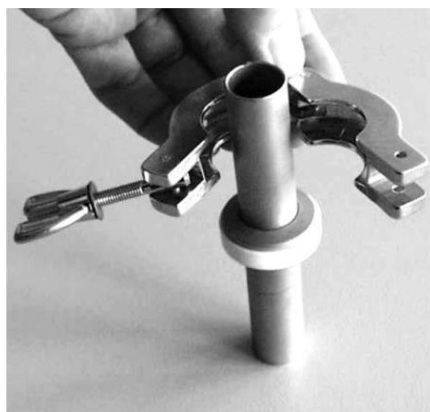
Fig. 69: Attaching the clamping ring
