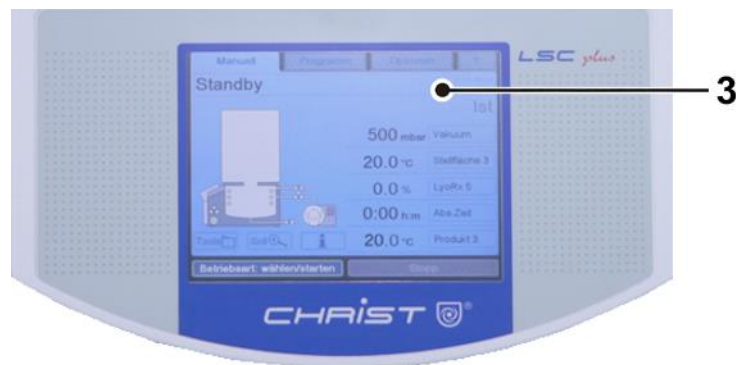
Fig. 74: User interface with touchpanel
