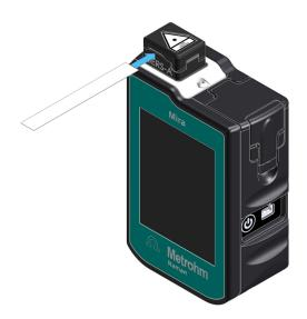
Slide the SERS paper substrate, **printed side down**, into the slot on the side of the attachment. Insert the strip until resistance is met. The attachment accommodates the strip at the optimal depth.
