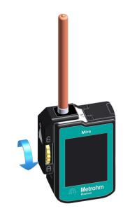
Tighten using the brass knob on the attachment. Do not over tighten.
