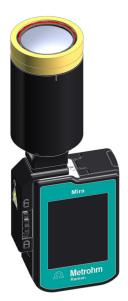
Manually adjust the adjustment ring to the desired Stand-off distance and acquire the data.
