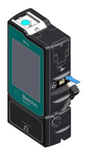
Connect the USB Mini-B plug to the instrument.
