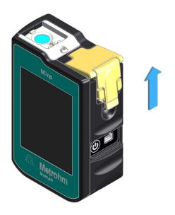
Push the lateral cover upwards.
