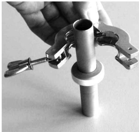
Fig. 53: Attaching the clamping ring
