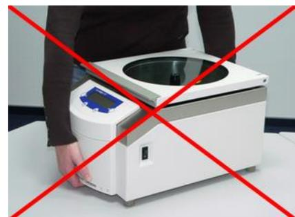
Fig. 6: Lifting the RVC
