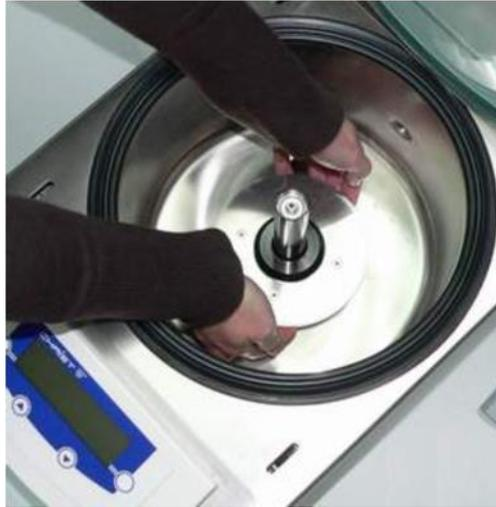
Abb. 57: Removing the rotor shaft
