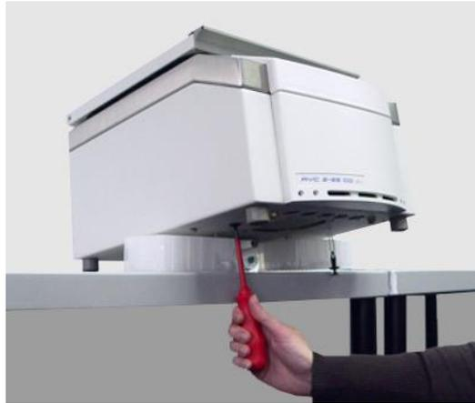
Fig. 48: Position of the unit over the edge of the table
