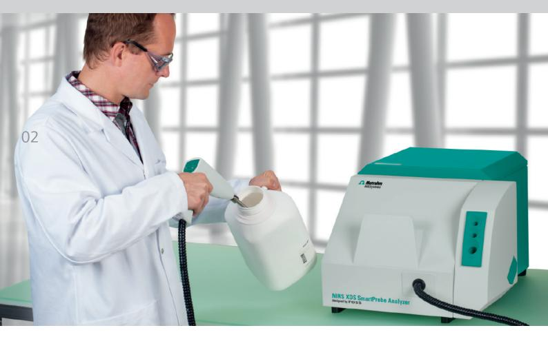
The NIRS XDS SmartProbe Analyzer enables fast, non-destructive analyses of solid and liquid substances and formulations. The NIRS XDS SmartProbe Analyzer can directly determine the identity and quality of a substance in its original transport containers; be it bottles, bags, or other containers. The anlyzer's robust and ergonomic design make the NIRS XDS SmartProbe Analyzer the ideal quality control solution in both the warehouse and in the laboratory.
