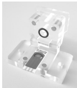
Figure 28: Flow cell (open) with electrode 6.1208.510
